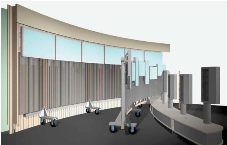
The curved collage of screens is mounted on a layered structure that nestles tight to the wall. For servicing, each of the three layers of screens and wiring harnesses pivots out from a single column.
