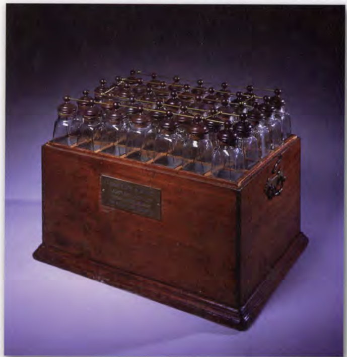
Figure 3. "Electrical battery" of Leyden Jars, 1760-1769. Franklin retired from the printing business in 1748 to focus on his civic and scientific interests. The publication in London in 1751 of Experiments and Observations on Electricity , a collection of Franklin's letters about the nature of electricity, brought him international recognition. American Philosophical Society
